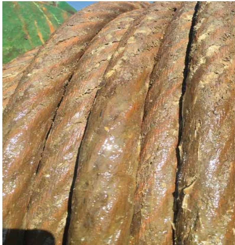
Extreme salt encrusted mud on a mooring rope
